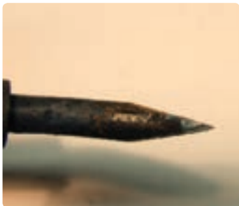
Oxidation on the tip of the soldering iron is removed by the use of soldering stone.
