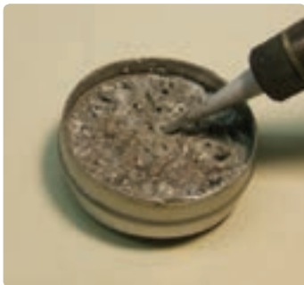
"Cladding" the tip of the soldering iron.
