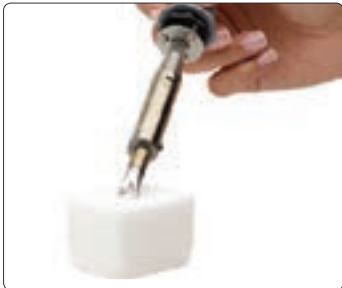
Cleaning the tip of the soldering iron with soldering stone.
