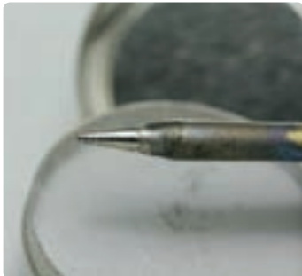
"Cladding" the tip of the soldering iron.
